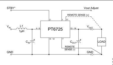
$\begin{array}{ll} C_{in} &= Required \ 1000 \mu F \ electrolytic \\ C_{out} = Required \ 330 \mu F \ electrolytic \\ L1 &= Optional \ 1 \mu H \ input \ choke \end{array}$
